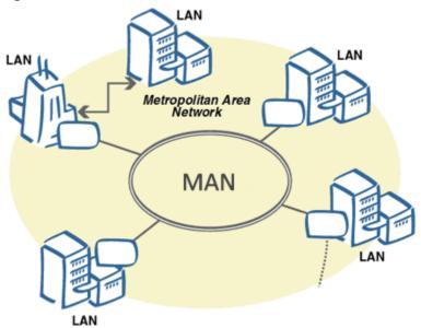
MAN is a high-speed network that spreads over a large geographical area such as a metro city or town. It is set up by connecting the local area networks using routers and local telephone exchange lines. It can be operated by a private company, or it may be a service provided by a company such as a local telephone company.
