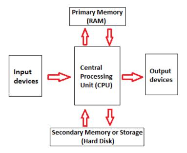
The operations of computer components are given below:
