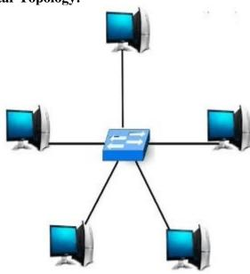
In this topology, all the computers are separately connected to a central node or connection point, which can be a server, a hub, a router, or a switch. This topology offers an advantage that if a cable does not work, only the respective node will suffer, the rest of the nodes will work smoothly. All data or messages that one node sends to another passes through the central hub.
